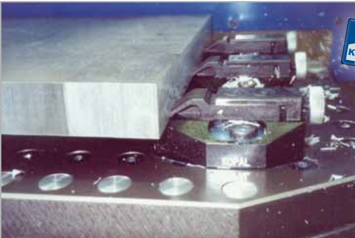
Machining of an aluminium plate with mini driving clamps on special supports
