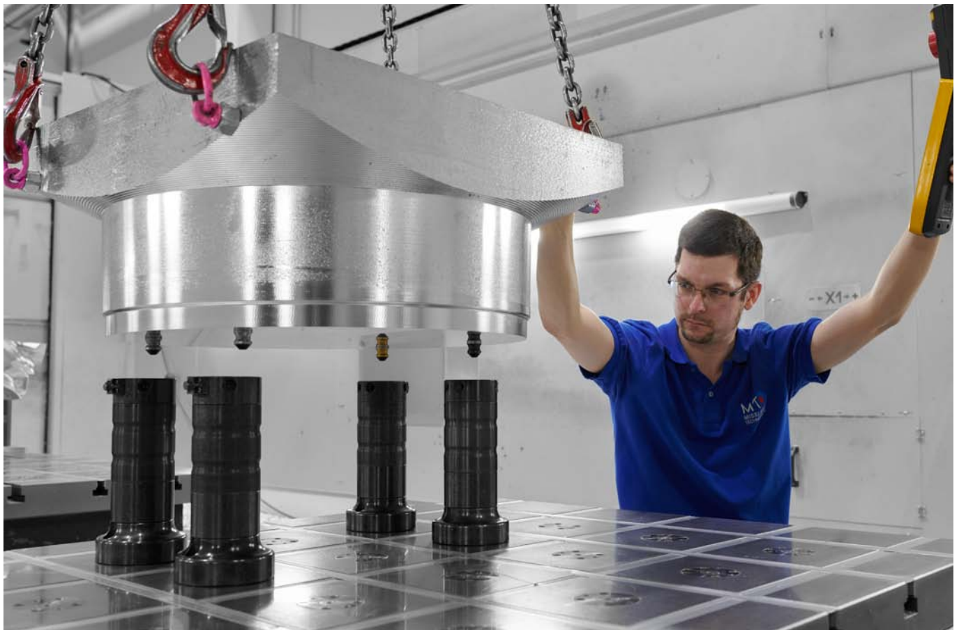
Minimize set-up times with AMF zero-point clamping technology: the workpiece is clamped in just a few simple steps for five-sided machining.
