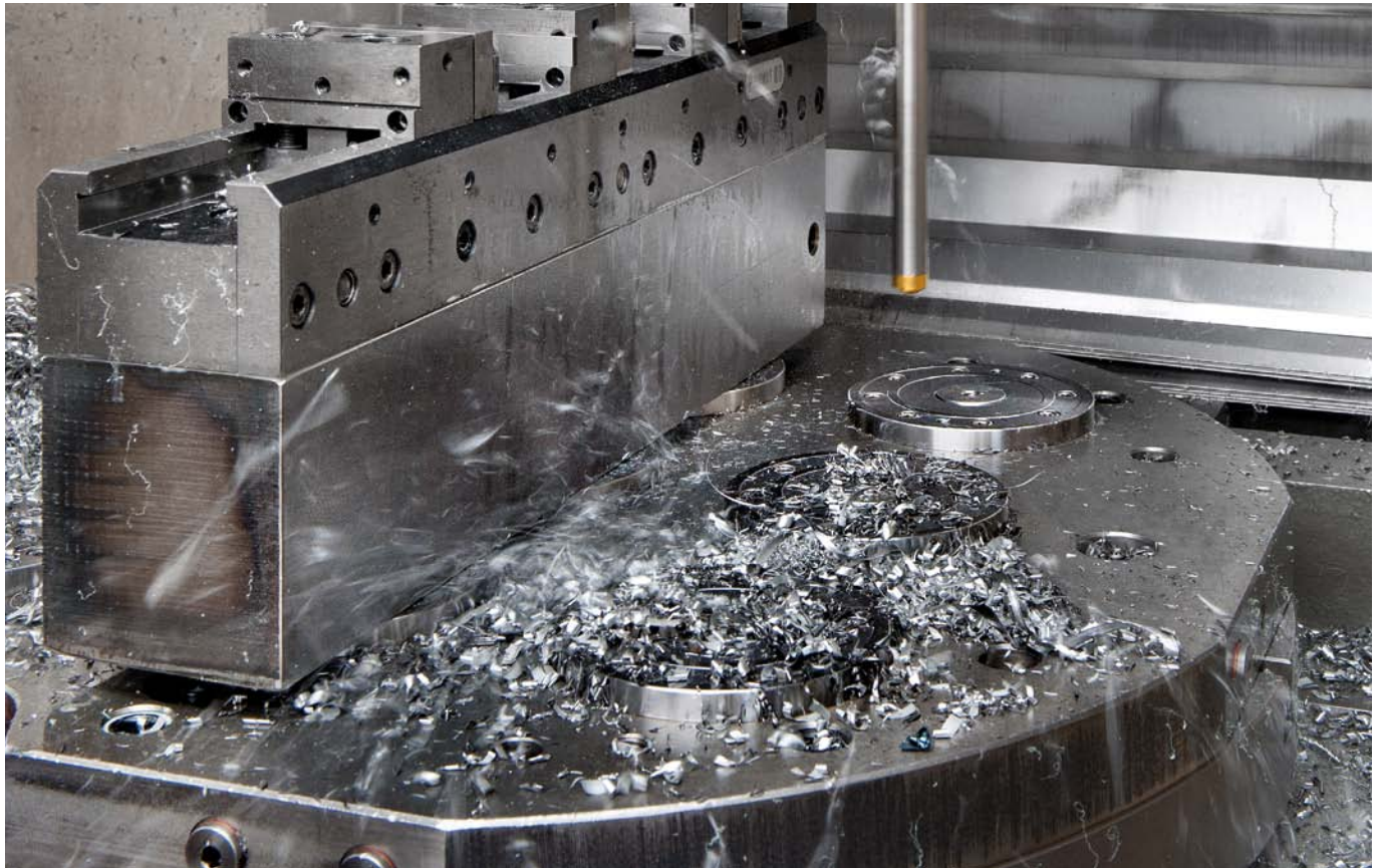
AMF-Clean-Stick in use: automated cleaning of clamping fixture and machine table.
