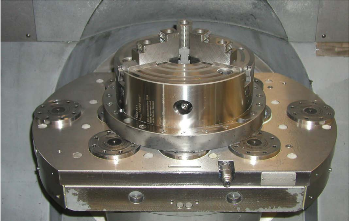
Simple changing of a 3-jaw chuck by means of the AMF zero-point system.
